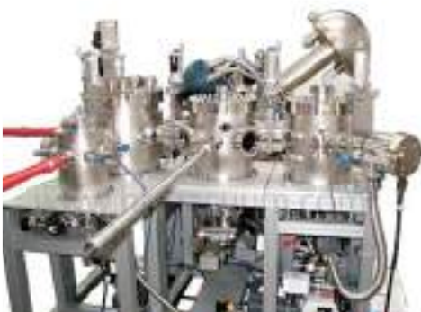
UHV System for Surface Analysis
